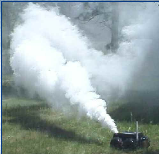
Smoke-Bot: Remotely Actuated and Delivered Tactical Concealment Obscuration and Riot Control Agent Dispenser Platform with FLIR
