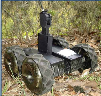
MITE: Upright or Inverted Mobility with Sensor Articulation and Automated Comms Recovery Behavior
