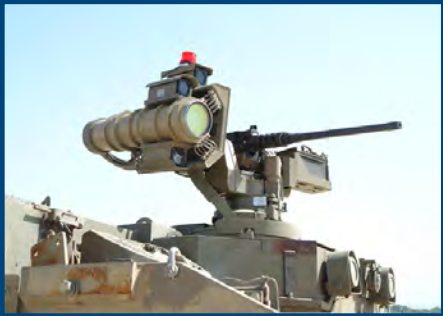
Articulated Pedestal with Laser Beam Director, Gun, Laser Range Finder and Aiming Cameras
