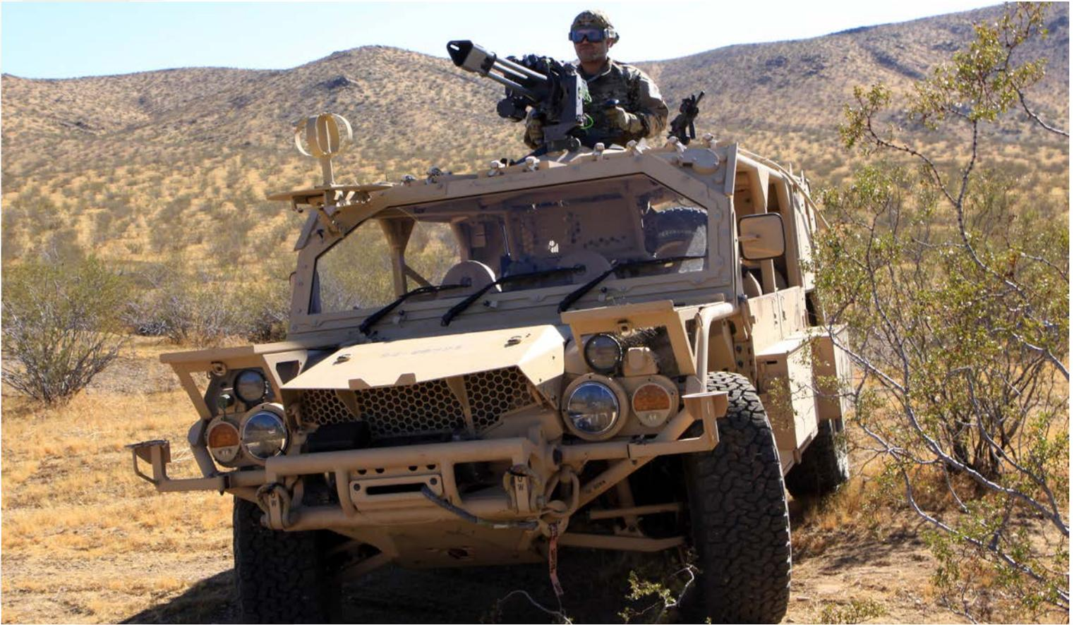
The Flyer<sup>®</sup> 72 is a non-developmental item, purpose-built, lightweight vehicle designed to meet complex mission sets. Selected by the U.S. Special Operations Command (USSOCOM) as the vehicle of choice for their Ground Mobility I.I (GMV I.I) program, at 72" wide it is capable of internal transport in the CH-47 and C-130 aircraft.
