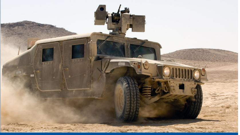
The Samson Mini is a high performance single-weapon remote weapon station designed for use with light combat vehicles and fast attack platforms. The dual axis, gyro-stabilized Mini has a low center of gravity for stabilization, making it the ideal remote weapon station for maneuvering forces. Armament can range from a 5.56mm machine gun up to 40mm automatic grenade launcher with an optional smoke grenade launcher.
