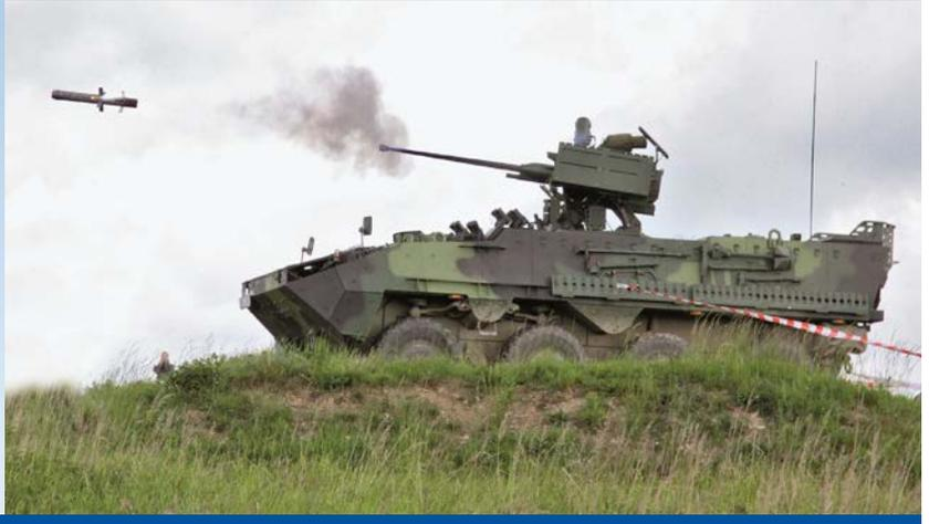
The Samson Mk I is a dual-axis, gyro-stabilized remote-controlled weapon system (RWS) capable of mounting multiple weapons. The retractable, dual-sighted Mk I supports main and secondary armaments, including a 25mm to 30mm main gun and a 7.62mm coaxial machine gun, as well as an optional anti-tank guided missile launcher and smoke grenade launcher.
