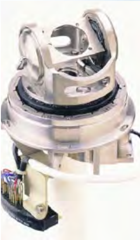
GDMS produces this 2-axis gimbal that can be used in a variety of applications. The gimbal consists of two brush type motors, a brushless motors, two resolvers, a slip ring assembly and the associated structural components and the electronics.
