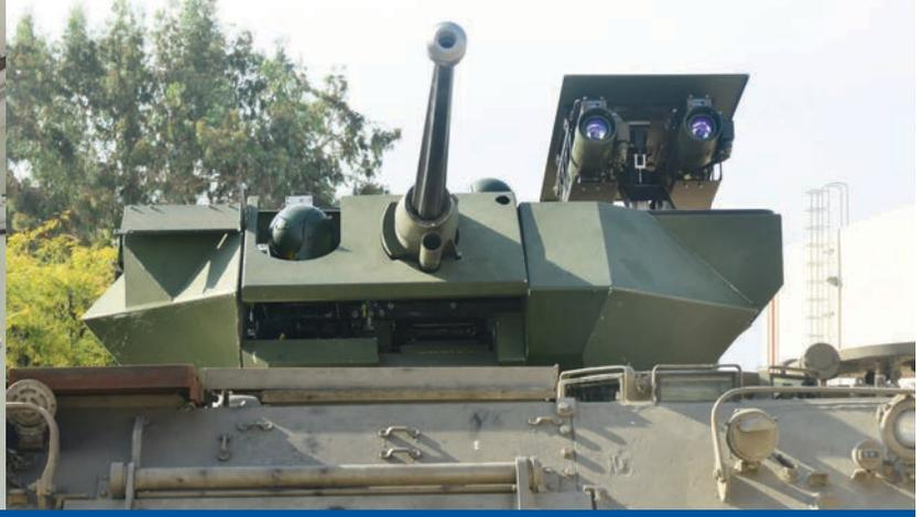
The Samson Mk II is a dual-axis, gyro-stabilized, dual-sight remote-controlled weapon system capable of mounting multiple weapons. Based on the Samson Mk I, the Mk II offers improved combat capability with a lower silhouette, optional armor protection, improved hit accuracy, under-armor reloading, increased rigidity and higher gun elevation capabilities.
