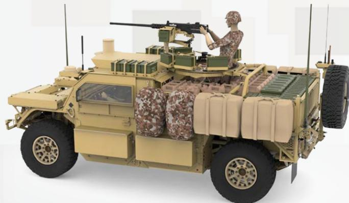
Manned or remote weapon station capable from 7.62mm to .50 caliber armament.
